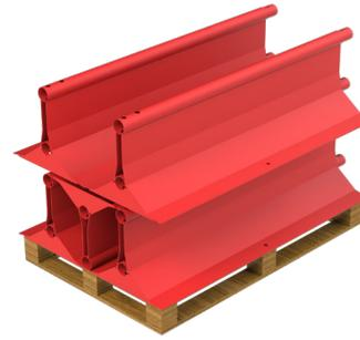
Carefully place a further two Manta Barriers side by side onto the previously placed pallet wood so that the inner edge of each foot touches the opposing barrier, each barrier should align top and side with the stacked barriers below.
